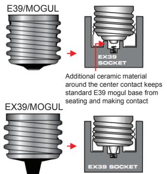
The EX39 base has an extended center terminal that can reach the center contact of an EX39 socket
